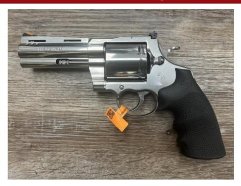
The Colt Kodiak features a 1-Piece full lug, ventilated rib stainless steel barrel with recessed target crown and ported for muzzle control. The leaf-spring action provides a non-stacking, smooth-as-glass trigger pull. Recoil-absorbing Hogue OverMolded rubber grips are interchangeable with all Colt Python and Anaconda grips. Unfluted 6-round cylinder chambered for 44 Magnum with a 4.25" barrel.
